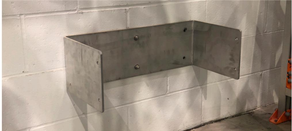
The LD421.280S Off Floor Mount Bracket must be mounted at the base of the ladder. It should be mounted a maximum of 3ft off the ground. Wherever possible, ensure that the mounting holes are not directly over a mortar joint.
